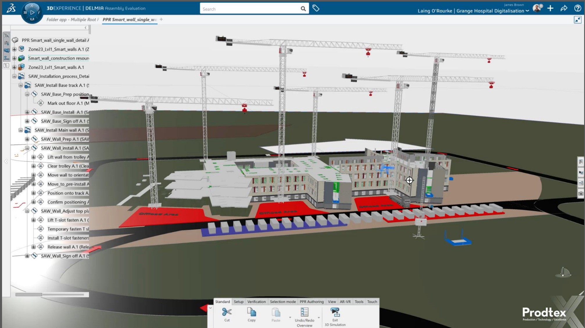
Proof of concept ergonomic assessment of Smartwall installation on The Grange Hospital design
